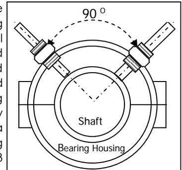
external access to the probe but allows the probe tip to be internal to the machine or bearing housing. **Advantages/Disadvantages:** Care must be taken in drilling and tapping the bearing housing or cover to insure that the probes will be perpendicular to the shaft center line. The benefits of this standard mounting include the ability to replace or adjust the probes without disassembly of the bearing and the location usually offers a good viewing area for the probe.
